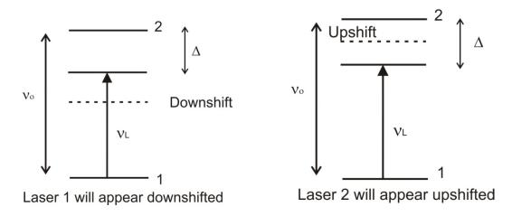
Differential absorption  $\rightarrow$  always more absorption from laser opposing motion causing motional damping
