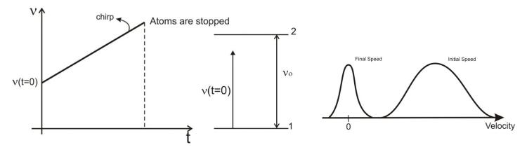
Atoms absorbing photons will be Doppler shifted So laser frequency is changed to keep laser on resonance Tune laser to correspond to most probable velocity from oven
