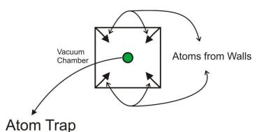
Source of atoms is within the chamber and cannot be turned off.
