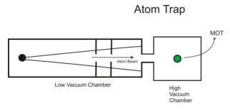
The source of atoms can be shut off by blocking the slit between vacuum chambers. The loss of trapped atoms is predominantly due to collisions with the background atoms. This results in an exponential decay of fluorescence modeled on the basis of the equation
