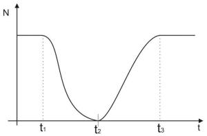
At t<sub>1</sub> the repump laser is turned off. The number of trapped atoms decays to zero. Once the repump laser is turned back on, the atom number reaches the steady state value.
